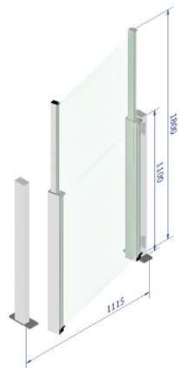
Wind Barrier wicket gate
